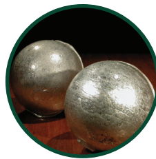
Cadmium Increases corrosion resistance of solders. Increases service temperature and strength of solder.
