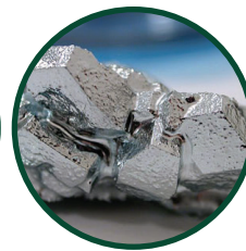
Gallium Has one of the longest liquid ranges for metals. Has low vapor pressure.
