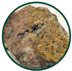
Gold Highly conductive and corrosion resistant. High melting point is reduced when alloyed with Sn, Si, or Ge.
