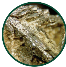
Bismuth Low melting when alloyed with Sn/Pb or In. Expands 3.32% on solidification. Non-toxic.
