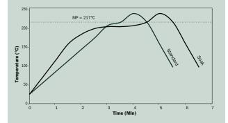
The stated profile recommendations apply to most Pb-Free alloys in the Sn/Ag/Cu (SAC) alloy system, including SAC305 (96.5Sn/3.0Ag/0.5Cu). This can be used as a general guideline in establishing a reflow profile when using **NC-SMQ®230** Solder Paste. Deviations from these recommendations are acceptable, and may be necessary, based on specific process requirements, including board size, thickness & density.
