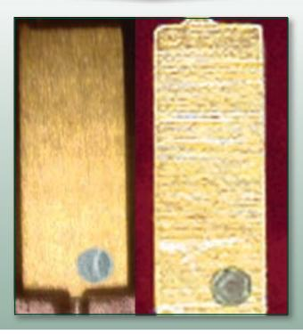
One major cause of flux and solder spatter occurs at the point of solder paste reflow. As the solder coalesces, it can cause flux remnant to "explode" outward and land onto nearby Au fingers. Solder paste fluxes designed with unique solvents and activators, such as **Indium5.8LS**, can provide a significant reduction in flux/solder spatter.
