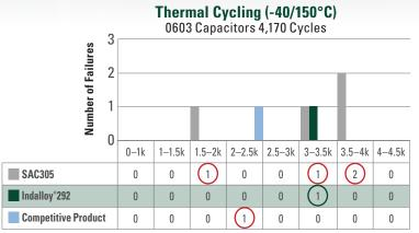
Indalloy® 292 has the least amount of failures (1) through 4,170 Cycles.
