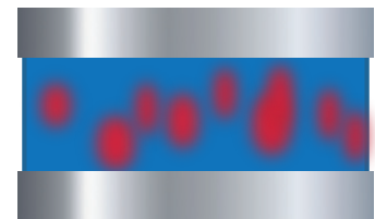
Fully Fused Solder Joint
