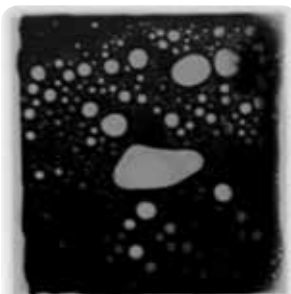
Typical Poor Voiding 10-12% Void Area
