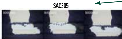
Massive cracking and complete failure on most joints at 3,000 cycles
