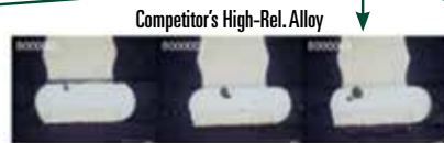
Inconsistent performance with some complete failures around 3,000 cycles
