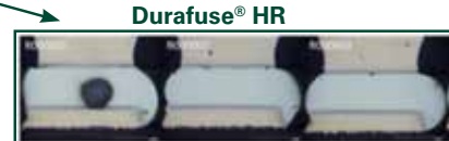
Minor cracking with zero failures up to 4,000 cycles
